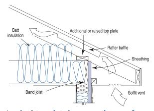
A raised top plate increases the area for insulation and ventilation at the eaves.
