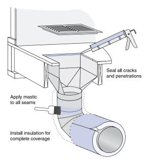
like quality, providing a permanent solution to unwanted leakage on both the return and supply side of the ductwork.
