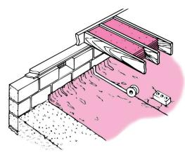
Insulate between the floor joists with R-19 batt insulation, making sure the paper side (vapor air retarder) is touching the underside of the floor, and that the insulation extends snugly against the band joist. Remember with paper-faced batts, the pink side should face toward the ground.
