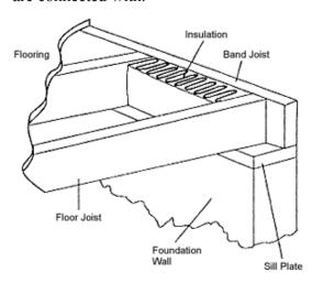
Cut 1- or 2-inch-thick foam board pieces to a rectangular size and insert between the floor joists, just above the foundation. Make sure to leave a ¼ inch gap around all sides. The edges are then sealed on all four sides with a bead of expanding foam.
